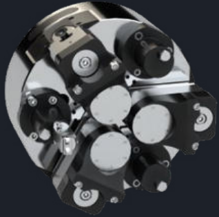
Cartridge lathe for gripping differential housing
